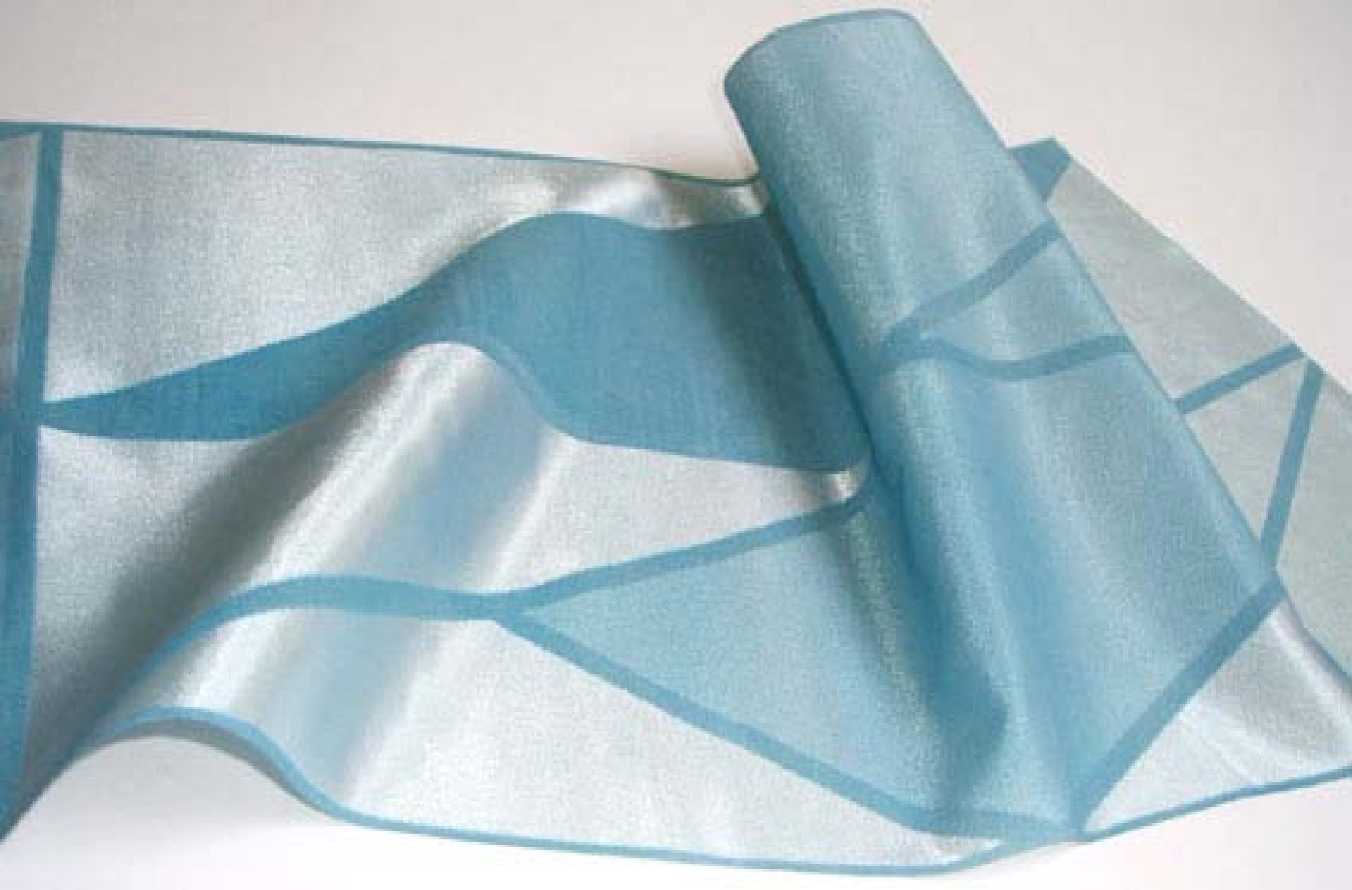
Laser processing affecting the shine of a satin weave
