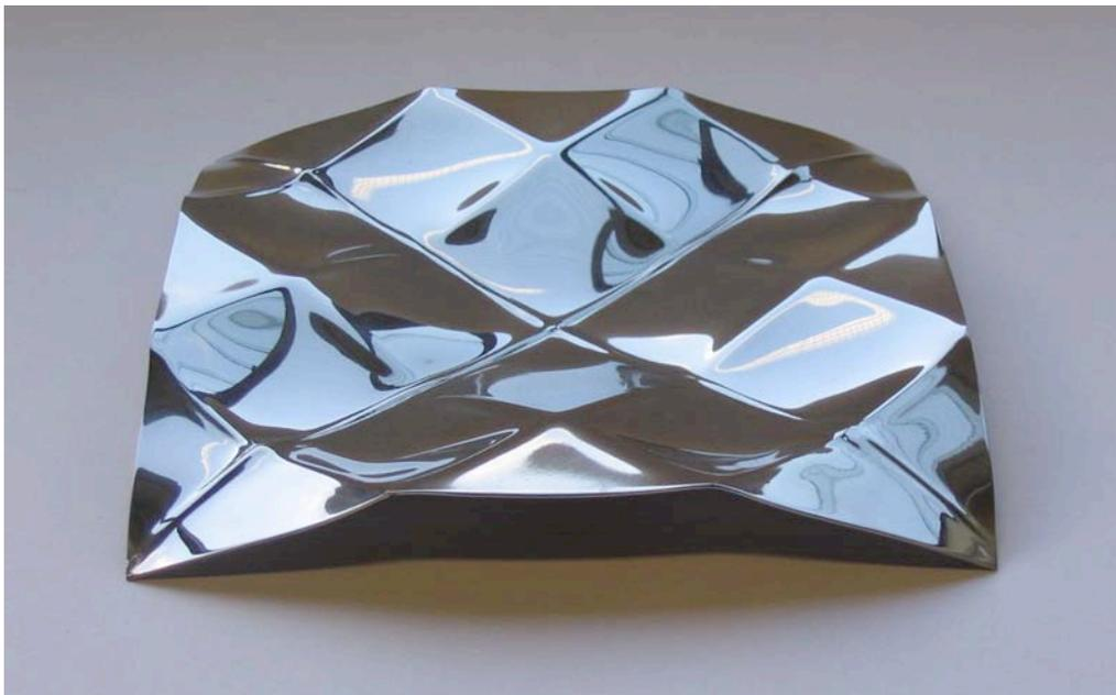
Figure 4: Dish formed by the positive and negative bending (buckling mechanism)
