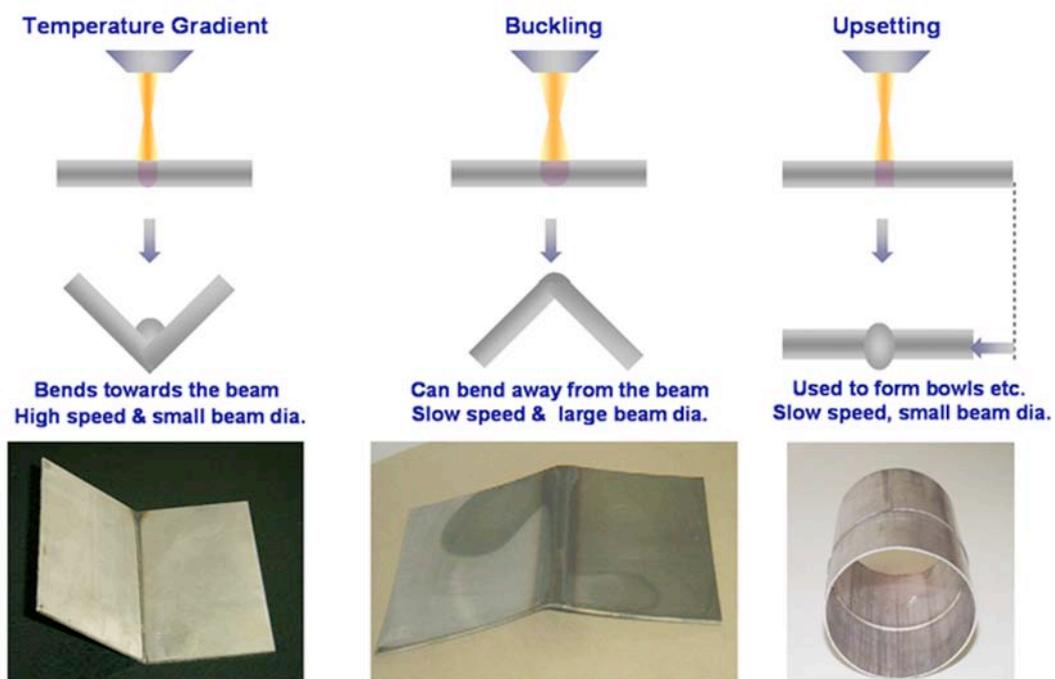
Figure 1: The heating scenarios for the three laser forming mechanisms.
