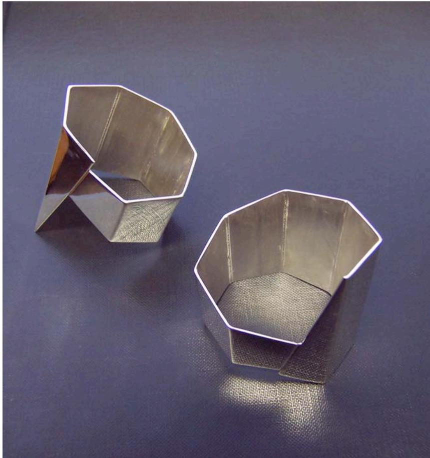
Figure 2: A pair of silver napkin rings, made by laser cutting and forming
