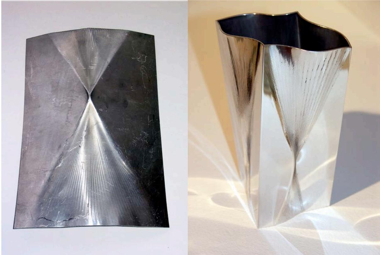
Figure 5: Vase formed from square tube, using the principle of a sheet experiment
